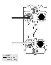
THIS MODULE MUST BE FITTED TO AN EARTHED FACE PLATE
