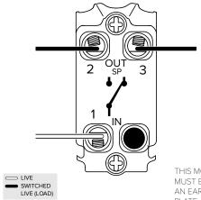
THIS MODULE MUST BE FITTED TO AN EARTHED FACE PLATE
