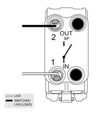
THIS MODULE MUST BE FITTED TO AN EARTHED FACE PLATE
