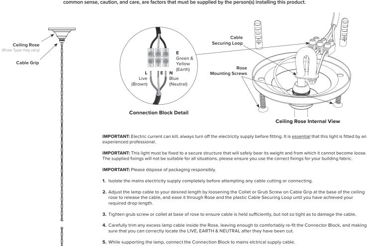
6. Fix the Rose to Ceiling (or other support surface) using the correct fixings for your substrate, ensuring that they are able to comfortably support the weight of the lamp.
